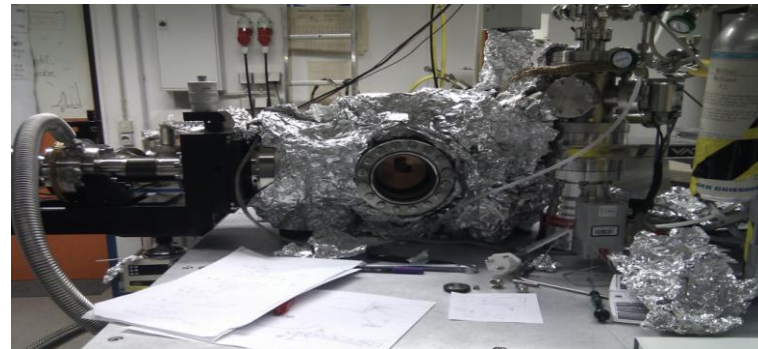
Figure 2. Set up of Thermal Desorption Spectroscopy
