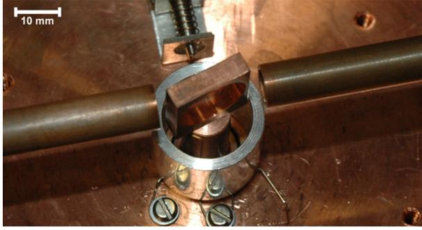
Figure 3: Pivot-mounted target frame in the collision volume (center). To the left and right of the target two cylinders are visible, within which the projectiles are accelerated from their storage compartments. In the center top of the image the target-release-mechanism can be seen, where the target can be lowered out of the collision volume during flight to allow for aggregate-aggregate collisions.
