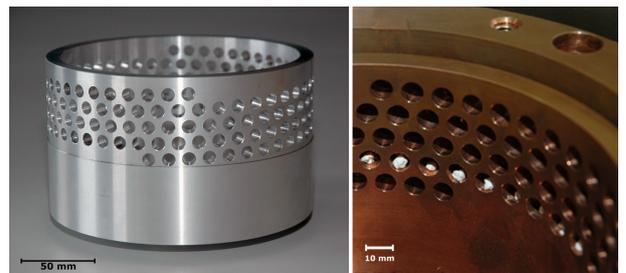
Figure 2: The cylindrical sample reservoir offers storage capacity for 180 individual millimeter-sized projectiles. On the left, the aluminum-made sample repository and to the right, the partly filled individual compartments of the copper reservoir.
