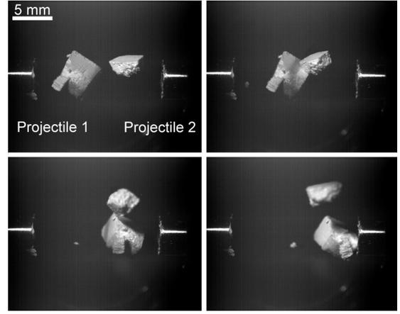
Figure 5: Example of a collision between two high-porosity dust aggregates. The collision velocity is  $\sim 0.4 \text{ m s}^{-1}$ . The time between subsequent images is 19 ms.
