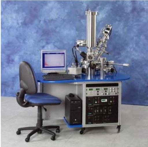
SurfaceSeer is a compact affordable TOF-SIMS designed for ease of use and speed of data acquisition. All the spectrometer tuning has been pre-set in the electronics, so that the surface chemistry of insulating, metals and semiconductor samples can be determined quickly and efficiently.
