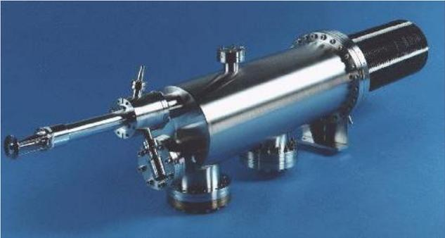
TOFSIMS add-ons based upon our R500 time-of-flight mass analyser with other components generally incorporated into "Do It Yourself" system builds for researchers aiming for a cost-effective route to obtain an instrument tailored to their particular requirements.
