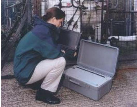
MS-200 is a portable, battery powered membrane inlet time-of-flight mass spectrometer for Volatile Organic Contaminants (VOCs) gas analysis.
