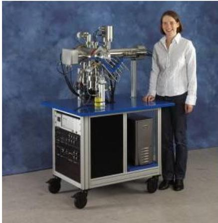
A Proton Transfer Reaction TOFMS for fast real-time high sensitivity analysis of VOCs in air. PTR sources selectively ionise VOCs from atmospheric pressure gas streams without ionising the major constituents of air. Therefore good at detecting trace levels of VOCs in complex chemical environments.
