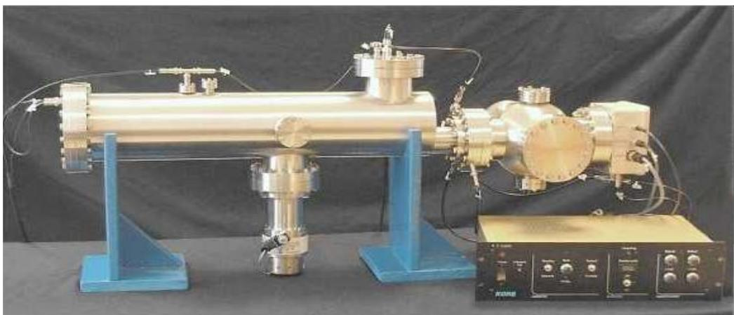
The Gas TOF-MS system is designed to add-on to experimental systems to provide mass analysis of a molecular gas stream. The mass spectrometer is used to characterise the masses and distribution of metal clusters produced in nanoscience experiments.
