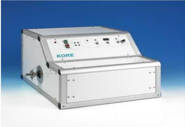
The Kore Fast Gas Analyser is a compact bench-top TOFMS providing rapid and sensitive gas analysis with the ability to produce stable long-term measurements of the constituents of gases at atmospheric pressures. The equipment is suited to process monitoring as well as catalysis studies and reaction kinetics research.
